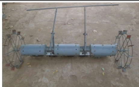
Fig. 2. Modified Drum Seeder.
