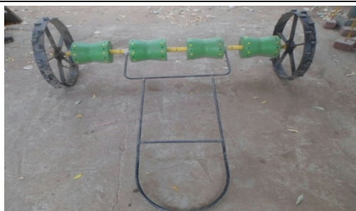
Fig. 1. Normal Drum seeder.
